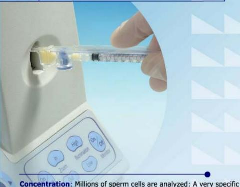
wavelength of light is absorbed by the sperm cells in the concentration chamber of the SQA-V testing capillary. An optical density detector measures the light absorbed by the cells. This is translated into cell concentration by a microprocessor based on a proprietary MES
